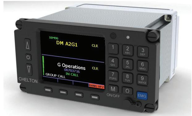
from the displays is LED white. Maximum NVIS radiance is within the MIL-STD-3009 published limits for 'multi-colour' electro-optical displays.
