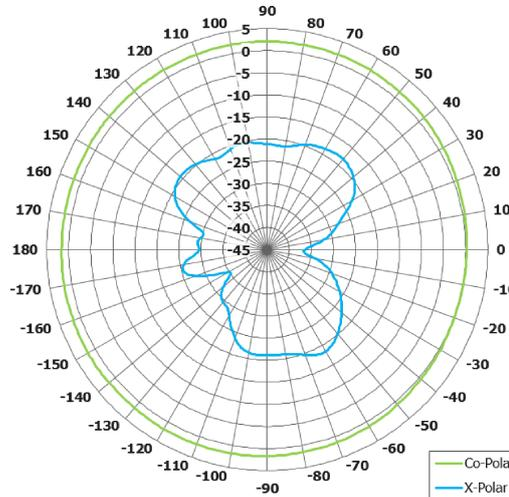
**Azimuth Polar Plot (@ 7.2 GHz)**
