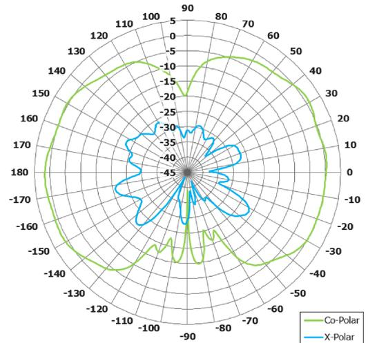
**Elevation Polar Plot (@ 7.2 GHz)**
