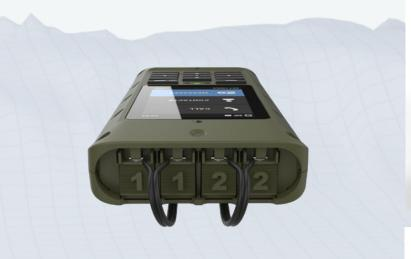
**Gateway** between CNR radio network and VoIP service
