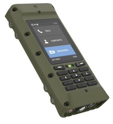
Chelton Tactical Gateway Interface (TGI) is a robust IP communication device designed for tactical networks. The device can be used for several purposes, such as SIP phone, router, and SHDSL modem, which makes it highly versatile for various field/tactical communication needs.
