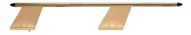
The 19-415 is an electrically small, high efficiency antenna, consisting of two glass reinforced plastic composite masts surmounted by an aluminium top loading. The antenna covers the VHF band 30 MHz to 88 MHz.
