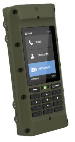
The device can be used for several purposes, such as SIP phone, router and SHDSL modem, which makes it highly versatile for various field/tactical communication needs.
